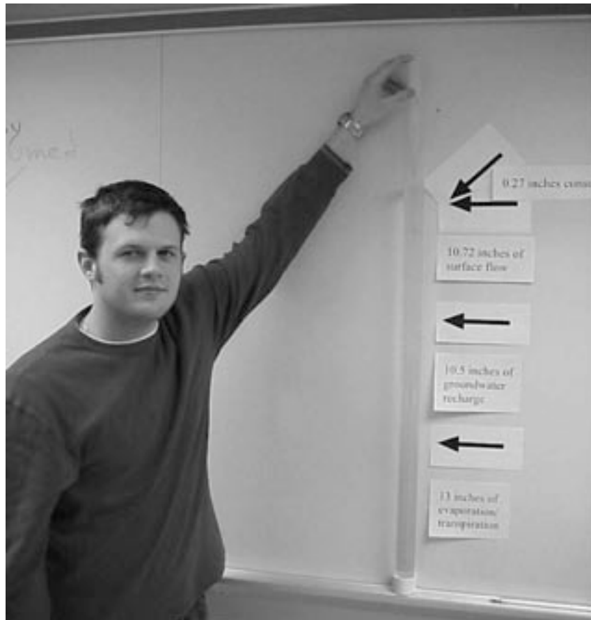
Figure 2. Using a cylinder of water as a visual scale of the components of the water cycle. The column of water is 34.6 inches high, the same as the precipitation in the watershed. Most of the water in the watershed is lost to evaporation/transpiration. About one-third of the water recharges groundwater or is discharged through surface water. A small percent is consumed. The relative amount of water bottled by Ice Mountain is about three one-thousandths (0.003) of an inch at this scale.
